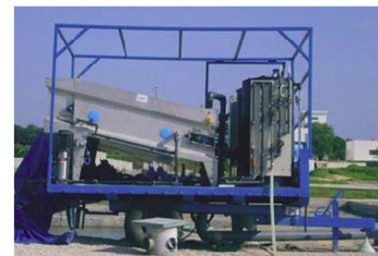
Mobile sludge thickening station before drying beds
