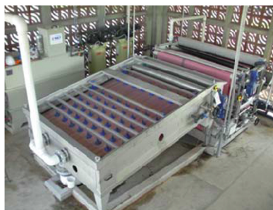
OMEGA 15 MD combined with belt filter press
